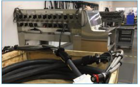
Each loop is computer tested on 12 Quality Assurance Points which are focused on Critical-to-Quality (CTQ) features.
