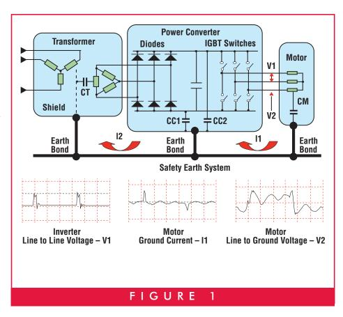
It is essential that the common mode currents return to the inverter without causing EMC - EMI problems in other equipment, and this means that the common mode currents I1 and I2 must not flow in the safety earthing system.
