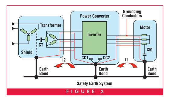
If symmetrical grounding conductors and an overall EMI shield are not used, EMC - EMI problems are very likely to occur.
